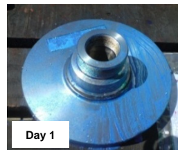
(Top) Fresh blue coating of Formula 60 Steelgard Rust Preventive on bonnet for one day.
