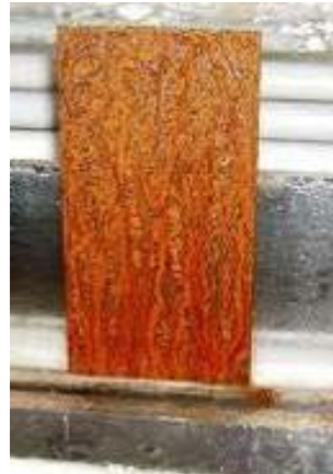
(Left) Reddish-brown rust appearing on an exposed iron plate.
